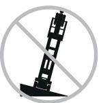
Do not depend on the tilt alarm as a level indicator. The tilt alarm sounds on the chassis only when the machine is on a slope.
